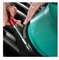
7. Once fully homed take a clamp of corresponding size and install it over the sleeve in the channel at the end of the boot. Use a T-Handle torque wrench to tighten the clamp to 60in-lbs.
