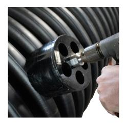
Take the hole saw of the corresponding size which has a pilot bit in it. Align the pilot bit into the hole in the valley.
